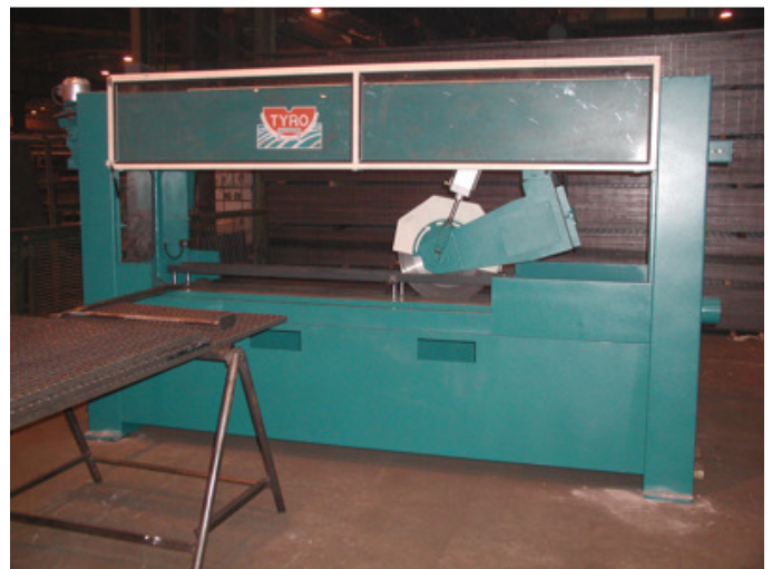
Special Clamping Beam with 3 cylinders for gratings cylinder to lift the head after the cut
